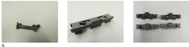
The shoe casting will have created a step in the back of the side frame, the bogie wing fits into this step. Put a small amount of glue onto the end of the bogie body wing and glue the bogie side frame into place. The wing should be lined up so it's exactly in the middle of the side frame, the wing and the back of the spring casting will line up and the brake shoe step will set the height.
